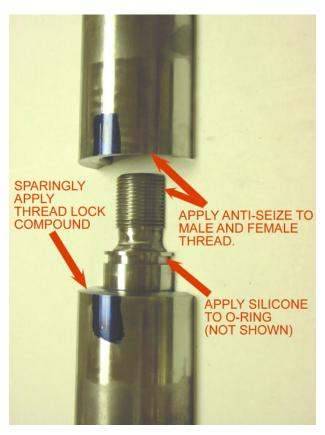
**10.** Apply anti-seize generously to both the male & female threads. <u>Do not</u> apply anti-seize to oring. Apply an o-ring safe silicone to the o-rings of the plunger and cylinder. Use a generous amount of silicone on o-rings, o-ring grooves, and immediate areas.
