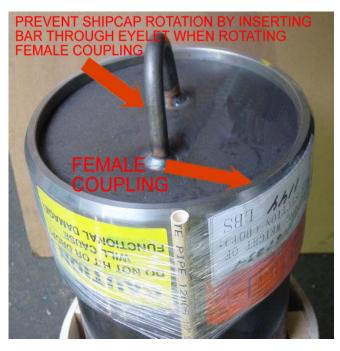
2. After the bottom section is securely mounted, remove female coupling with spanner wrench or strap wrench to expose plunger for installation of the next jack section. The female coupling is removed in a counter clockwise rotation. When removing the female coupling secure the eyebolt with a bar. This will prevent the eyebolt from turning with the female coupling. NOTE: Do not unscrew top shipcap at eyebolt because it may jamb shipcap, damage plunger or plunger coupling.
